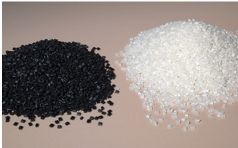
Abrasive reinforced polypropylene resins caused wear and failure of traditional long-sweep pneumatic elbows. Impact of material against the elbow wall also created fines and frictional heat that partially melted the resin.
