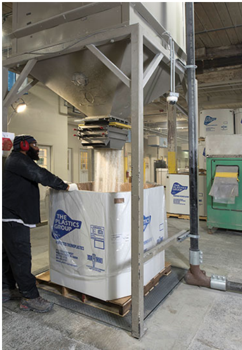
The Plastics Group conveys approximately 3,300 lb (1,497 kg) per hour of reinforced resins through two pneumatic lines, and between 1,200 to 1,500 lb (544 to 680 kg) per hour through a third line.
