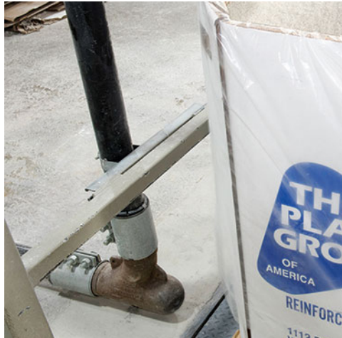
The Plastics Group replaced conventional sweep elbows with HammerTek deflection elbows, none of which has needed replacing. By preventing material impact with the elbow wall, the company has prevented elbow wear, the generation of fines and the frictional heat that previously caused the formation of angel hair and streamers.
