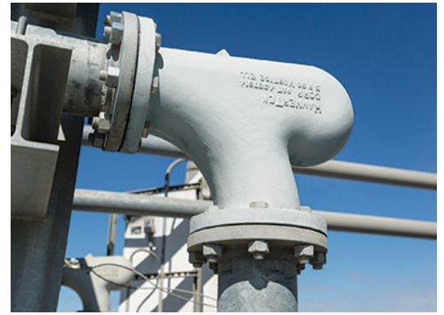
The teardrop-shaped vortex chamber designed into the curve of the Smart Elbow creates a deflection zone that minimizes elbow wear and product degradation without compromising material flow.
