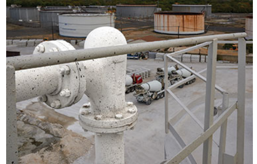
Action Supply, Sharon Hill, PA, eliminated surprise blowouts and associated repair costs after switching to short radius deflection elbows that minimize elbow wear.
