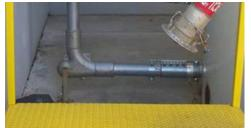
On system start-up, a gently rotating, self-renewing ball of material is formed in the vortex chamber, causing a change in conveying direction though deflection.
