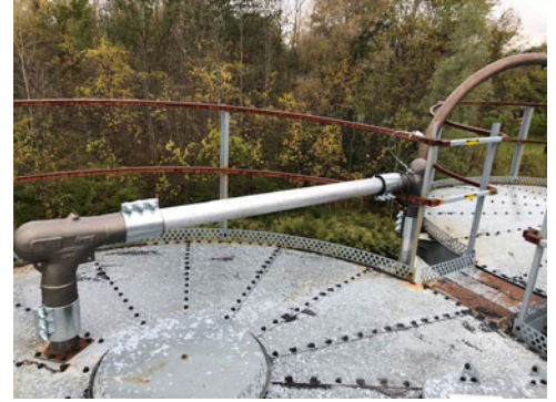
At Parker Chomerics, two 90-degree deflection elbows from HammerTek eliminated elbow wear previously experienced with stainless steel sweep elbows, ceramic lined elbows, ceramic backed elbows, and elbows fabricated in-house using flexible stainless steel pipe and quick-connect fittings.
