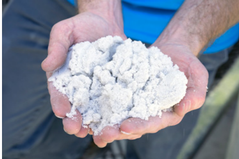
Sand, a raw material for Ardex Americas' engineered cements, adhesives, and high-performance building products, severely abrades pneumatic pipelines.
