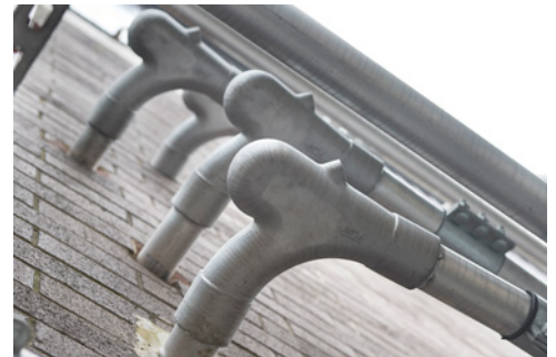
The Smart Elbow® design prevents PE pellets from impacting/heating the elbow wall, melting and forming streamers.
